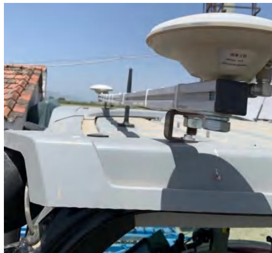
Figure 2.15 Installation example of dual-antenna – 2
