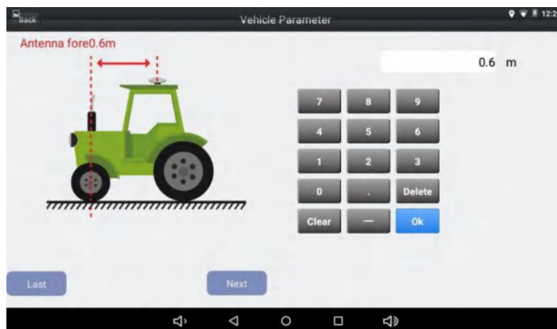
Figure 2.33 Vehicle parameter configuration – antenna fore
