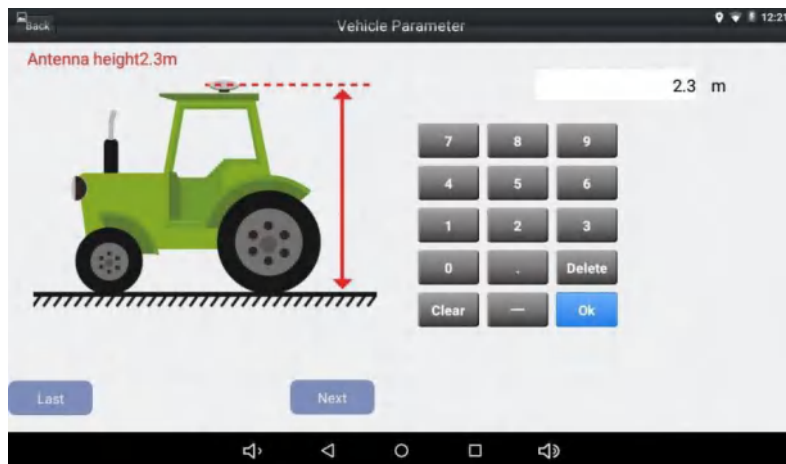
Figure 2.30 Vehicle parameter configuration – antenna height
