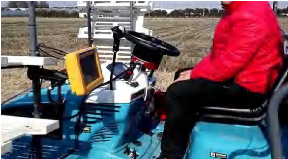
Figure 5.3 Transplanting using JY302 auto-steering system
