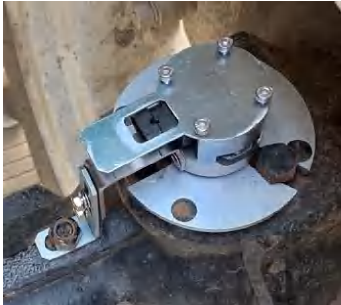
Figure 2.10 Fix angle sensor – 2
