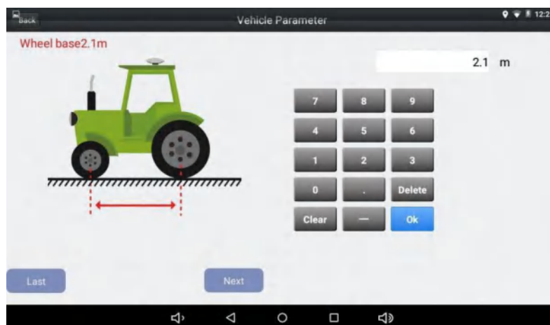
Figure 2.34 Vehicle parameter configuration – wheelbase
