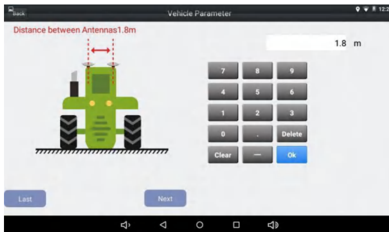
Figure 2.32 Vehicle parameter configuration – antenna distance
