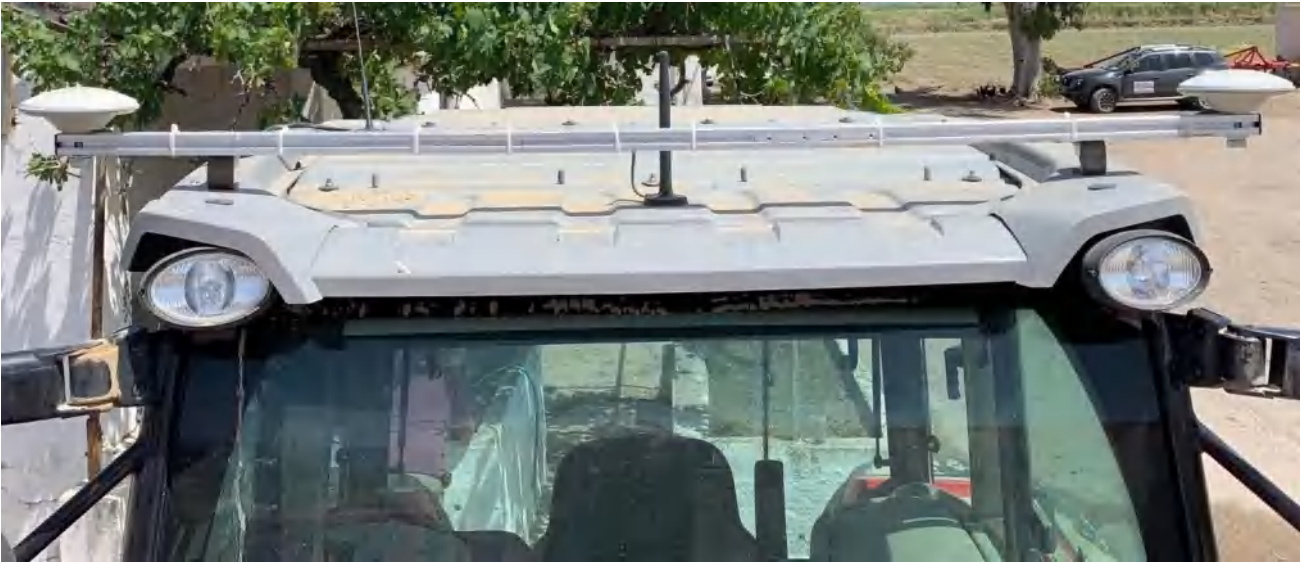
Figure 2.14 Installation example of dual-antenna – 1
