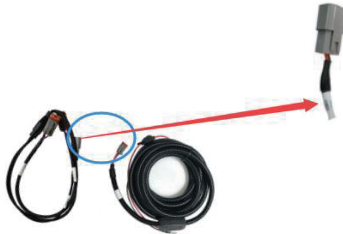
Figure 2 Power supply cable - main harness
